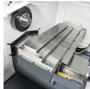
XZ axes BOX guideway with precise scrapping
