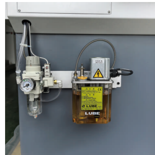
SMC pneumatic parts and LUBE lubrication pump
