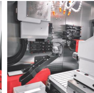
CSL076 with back spindle(Z2 axes)
