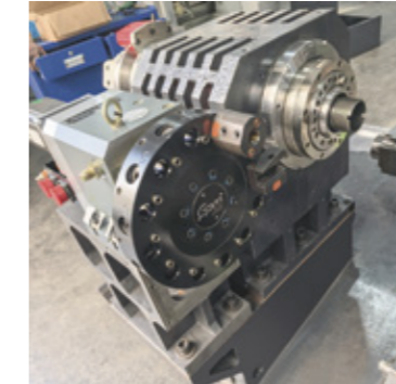
Left VDI20 Hydraulic servo tool turret (non-powered)
