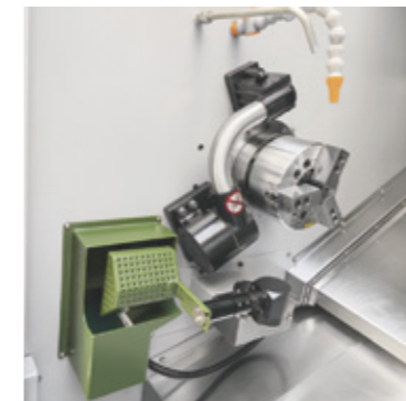
Tool setting probe and parts catcher
