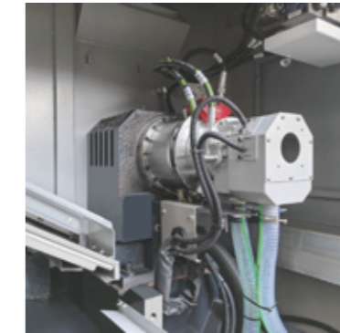
CS axes with hydraulic brake
