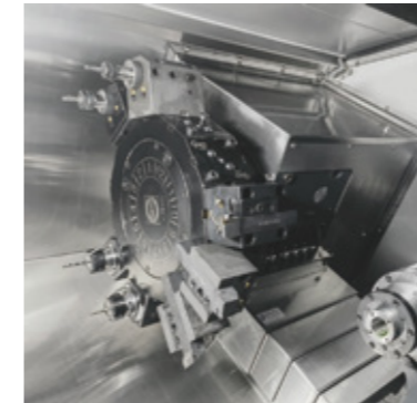
SAUTER(GPM) 12T powered tool turret
