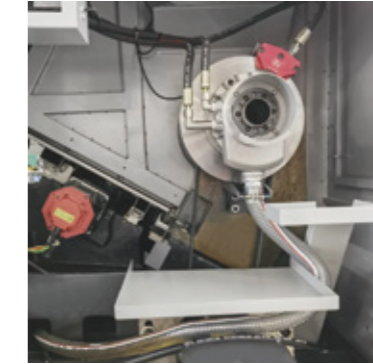
CS axes with hydraulic brake
