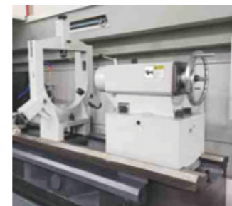
Strong tailstock and steady rest
