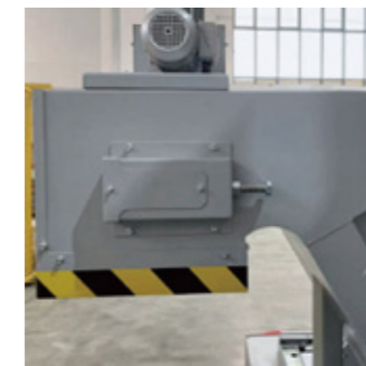
Widened & thickened chip conveyor
