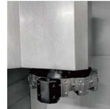
VL400 600 800 1000 12T hydraulic-servo turret
