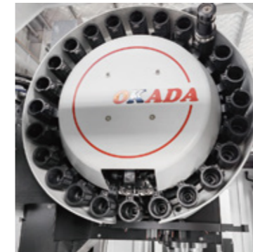
24T ARM type tool magazine
