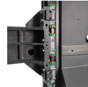
V8 V11 Z axes 6 slide blocks
