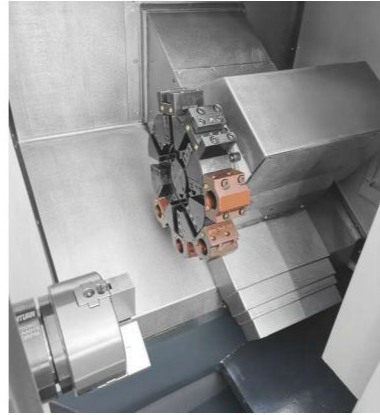
S32T mount chuck+8T servo tool turret
