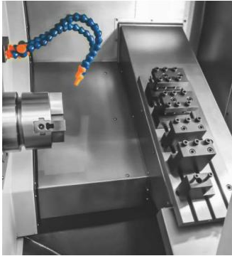
3-jaw chuck with gang tool
