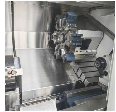
S200 200L own-made 12T hydraulic-servo turret
